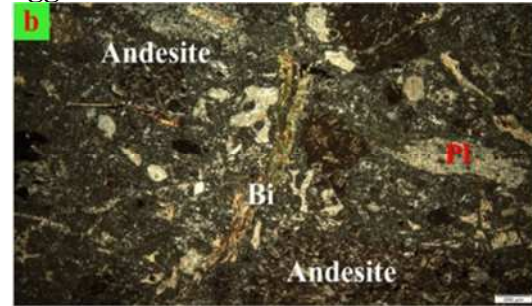
Fig. 73: Crystal fragments of the biotite (Bi) and plagioclase (Pl) with several lithic fragments of andesite in lithic crystal agglomerates.
