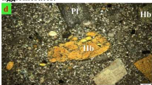
Fig. 75: Crystal fragments of altered hornblende (Hb) and plagioclase (Pl) with iron oxide inclusions in crystal agglomerates.
