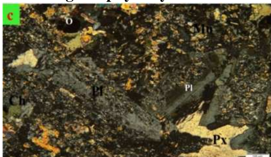
Fig. 93: Crystals of partially altered plagioclase (Pl), muscovite (Mu), pyroxene (Px) and opaques (O) in basic diabase dyke.
