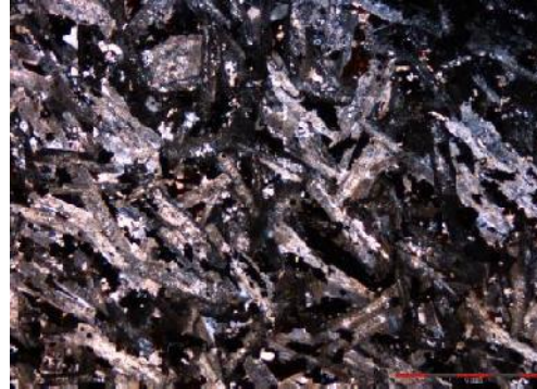
Fig. 8: Microscopic photo showing parallel alignments of quartz and feldspars forming directive texture in trachyte
