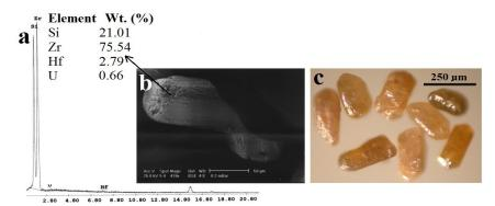
Fig. 5: Coloured zircon crystals EDX analysis (a), ESEM backscattered image (b) and zircon crystals under binocular microscope (c), X = 10.
