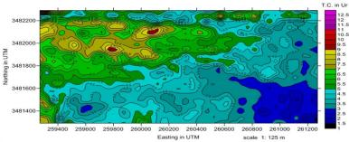
Fig. 7: Ground radiometric distribution contour map of total count in  $\left(\mu R\right)$ of the study area
