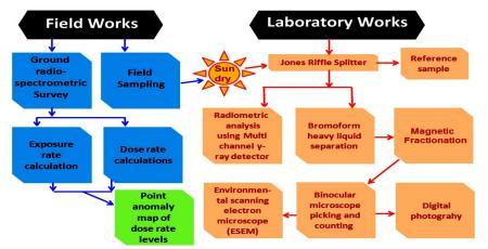
Fig. 3: Flow sheet showing the methods applied to the present study
