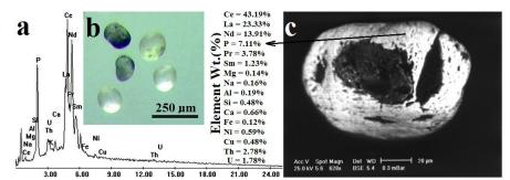
Fig. 6: EDX analysis (a), binocular microscope (X = 20) photo of monazite crystals (b) and ESEM backscattered image (c).
