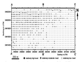
Fig. 16: The point anomaly map of the different dose rate levels at the different stations (50 m in-betweens) of the study area in mRem/y. The three profiles (A-A`, B-B` and C-C`) were used to collect field borehole samples
