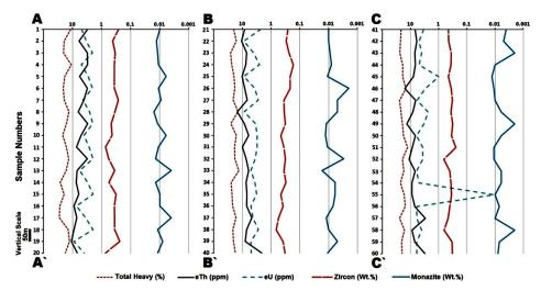
Fig. 17: Lateral variation diagram of zircon (%), monazite (%), eU (ppm) and eTh (ppm) across A-A', B-B' and C-C' profiles in the studied area
