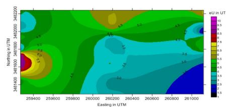
Fig. 11: The subsurface eU levels (to depth 0.5 m) from laboratory sample analysis
