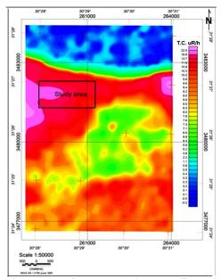
Fig. 2: Total count ( $\mu$ R) aeroradiometric coloured contour map of the area under study and surroundings, modified (After El Sirafy, et al., 2002)
