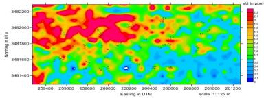
Fig. 9: Ground radiometric distribution contour map of eU(ppm) of the study area
