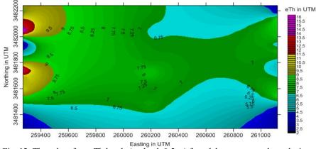
Fig. 12: The subsurface eTh levels (to depth 0.5 m) from laboratory sample analysis
