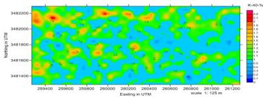
Fig. 8: Ground radiometric distribution contour map of potassium % of the study area
