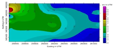
Fig. 13: The subsurface Radium (eU) levels in the depth of 0.5 m from laboratory sample analysis
