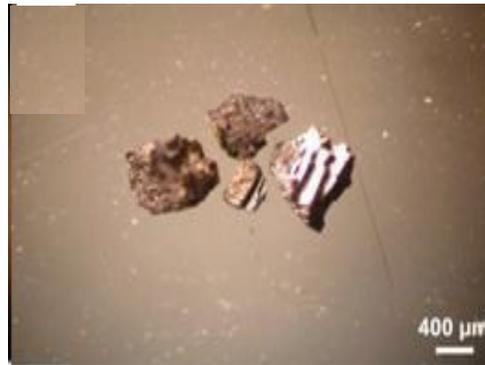
Fig.42: Galena grains from altered monzogranite,
