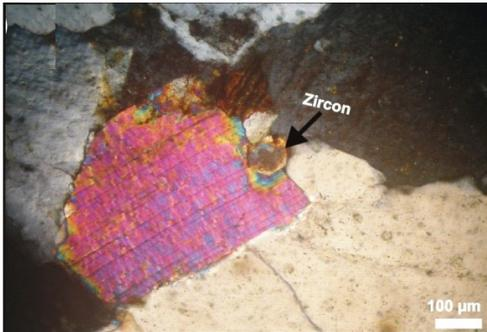
Fig.10: Photomicrograph showing zircon crystal associated with muscovite and biotite in monzogranite, XPL
