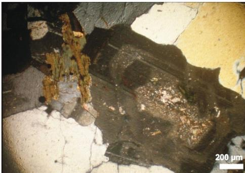
Fig.6: Photomicrograph showing chloritized biotite protruding the zoned saussuritized plagioclase in monzogranite, XPL
