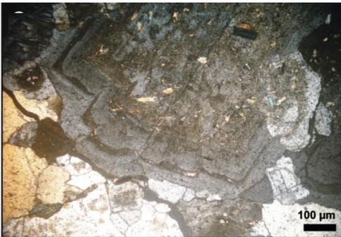
Fig.5: Photomicrograph showing large zoned crystal of saussuritized plagioclase in monzogranite, XPL
