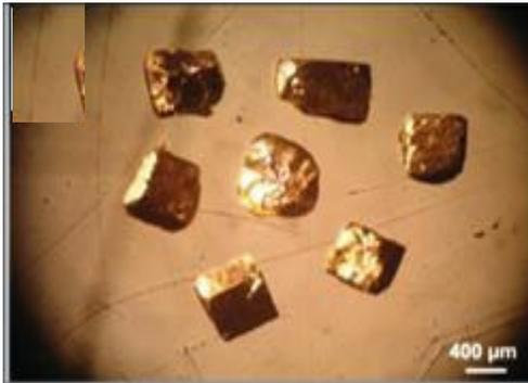
Fig. 39: Pyrite grains from altered monzogranite
