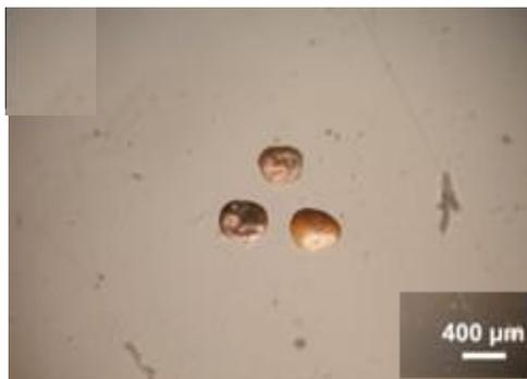
Fig.44: Hematite grains from altered monzogranite
