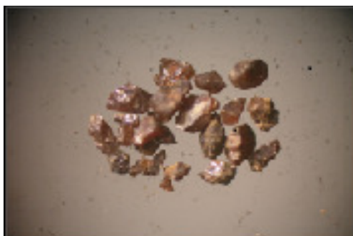
Fig.25: Photomicrograph of some dark brown to black grains of cassiterite mineral in Ras Baroud pegmatite body
