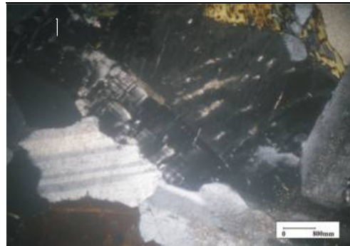
Fig.9: Subhedral crystal of microcline associated with plagioclase and perthite, XPL
