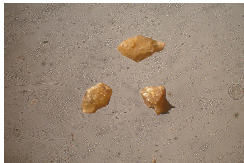
Fig.27: Photomicrograph of some malacon type zircon grains with greyish to yellowish green color in Ras Baroud pegmatite body
