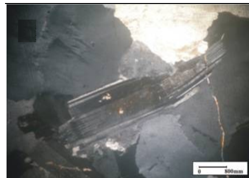
Fig.11: Deformed plagioclase with sericitization, XPL
