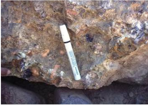
Fig.6: Illitization and fluoritization in the studied pegmatite
