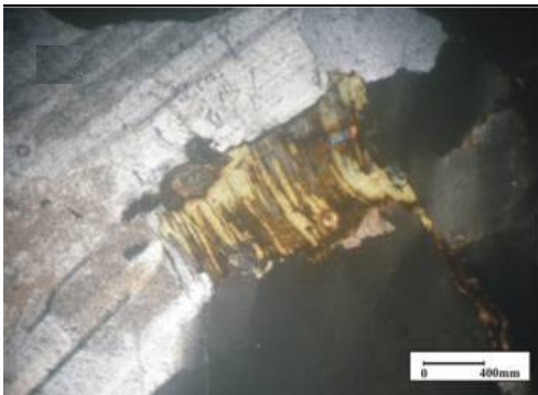
Fig.14: A flake of chloritized biotite including zircon, quartz and plagioclase, XPL
