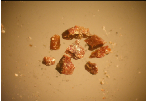
Fig.21: Photomicrograph of some reddish brown to dark brown grains of samarskite-Y mineral in Ras Baroud pegmatite body
