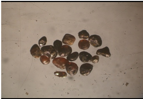
Fig.30: Photomicrograph of rutile grains with different colors
