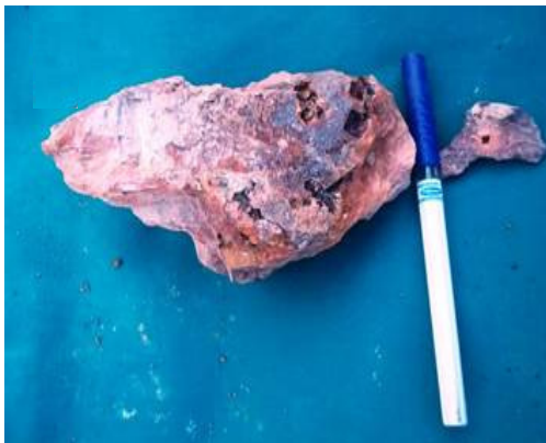
Fig.7: Hematitization in the studied pegmatite
