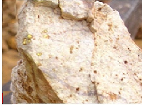
Fig.6: Visible uranophane fill the vugs of dissolved pyrite in silicified and albitized samples (Alteration process)
