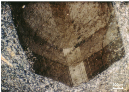
Fig.10: Normal zoned plagioclase phenocrysts showing alteration decreasesg from core to the outer rims in parallel to An-content,XPL
