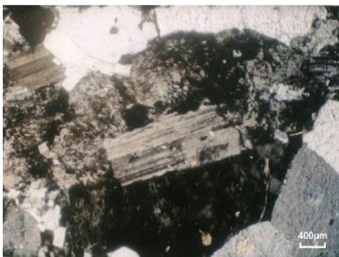
Fig.26: Albite and Carlsbad twinned fresh plagioclases, XPL
