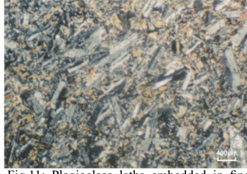
Fig.11: Plagioclase laths embedded in fine grained groundmass with random orientation forming typical pilotaxitic texture, XPL
