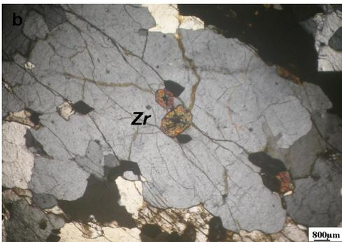
Fig.11:Quartz of the granitic fragment corroded by the finer quartz and encloses zircon , XPL
