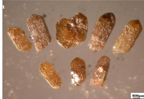
Fig.32: Stereophotograph of zircon separated from the anomalous rock of Wadi Ras Abda., long prismatic zircon crystals.
