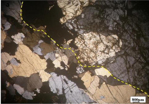
Fig.10:Boundary of the granitic fragment (dashed line) in contact with the finer quartz, XPL
