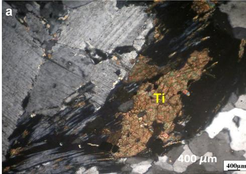
Fig.6:Photomicrograph of the granodiorite surrounding the anomalous rock showing: secondary titanite (*Ti*) associating penninite, XPL
