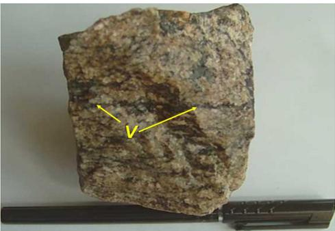
Fig.4: Close up view of Ras Abda granodiorite enclosing black veinlets (V) squeezed from the silicic magma
