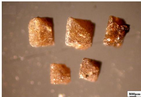
Fig.34: Stereophotograph of zircon separated from the anomalous rock of Wadi Ras Abda., Short prismatic zircon crystals.
