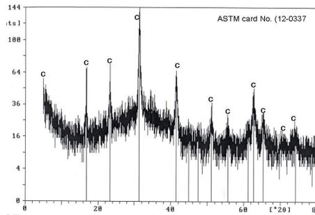
Fig.42: XRD-diffractogram of the columbite
