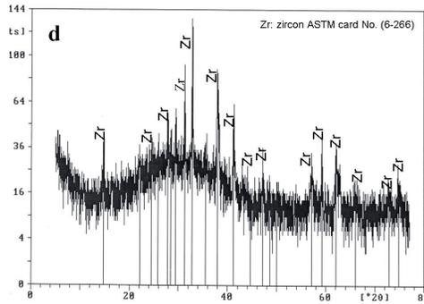
Fig.35: XRD diffractogram of zircon
