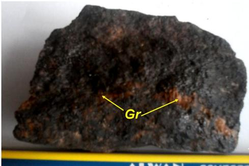
Fig.3: Close up view of the quartz vein enclosing granitic fragments (Gr) from the wall rock
