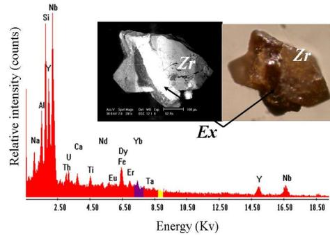
Fig.49:Stereophotograph, BSE image and EDX of euxenite intergrowth with zircon from the anomalous quartz vein of W. Ras Abda
