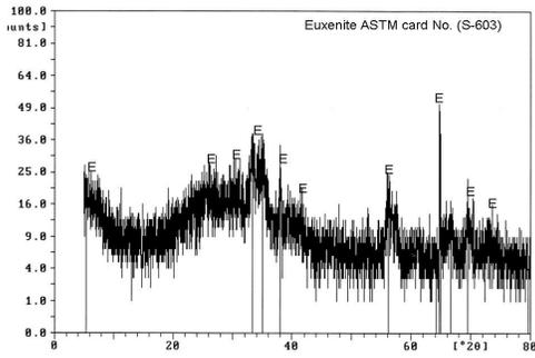
Fig.46:XRD-diffractogram of Euxenite after heating of the uranopolyrase (950°C)
