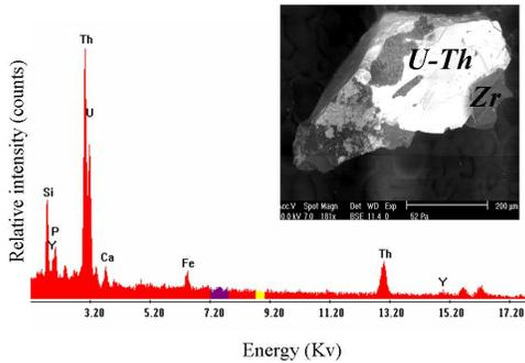
Fig.39: BSE image and EDX of uranothorite inclusion from anomalous quartz vein
