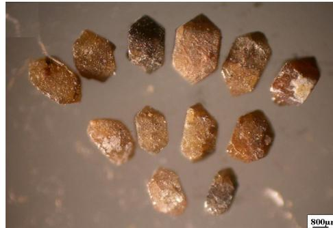
Fig.33: Stereophotograph of zircon separated from the anomalous rock of Wadi Ras Abda, Medium prismatic zircon crystals
