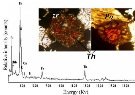
Fig. 38: EDX and Photomicrograph of thorite (Th) inclusion in zircon and uranopolyrase crystal (Po).
