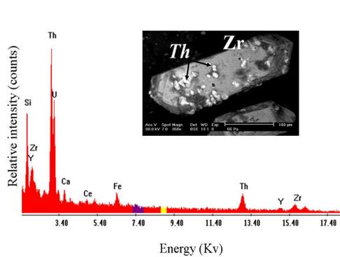
Fig.37:BSE image and EDX inclusions of uranothorite (Th) in zircon (Zr) crystal
