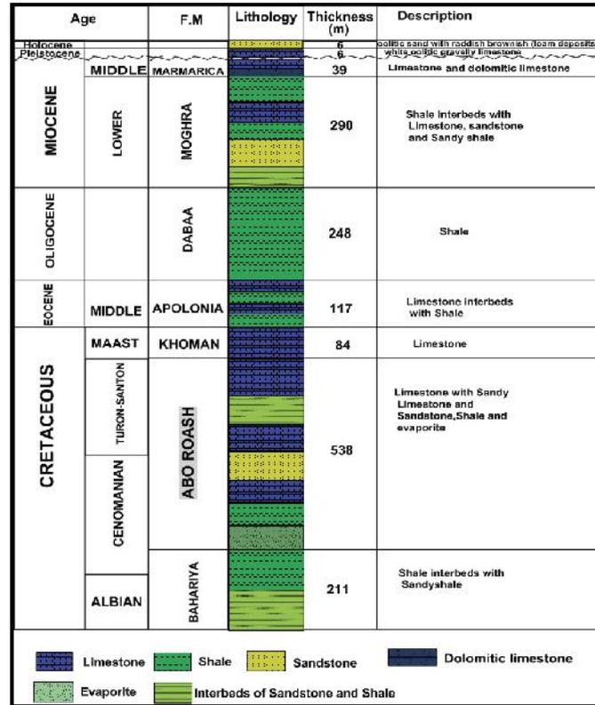
Fig. 6: Stratigraphic columnar section of the study area (After Sofratome, 1984)
