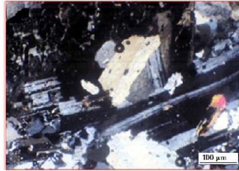
Fig.15: Photomicrograph shows the component of syenogranite; K-feldspar, quartz, plagioclase, biotite flakes and zircon
