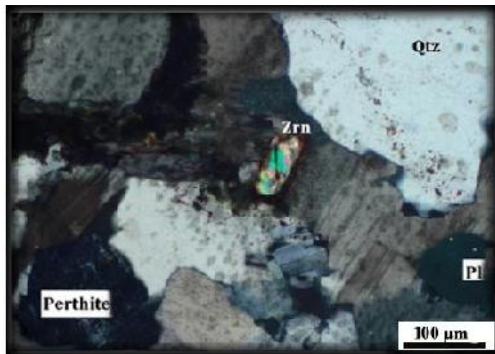
Fig.14: Photomicrograph shows the components of monzogranite; quartz (Qtz), K-feldspar (Perthite), plagioclase (pl) and zircon (Zrn).
