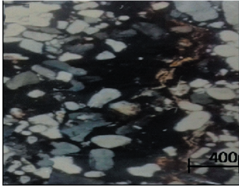
Fig. 9: Photomicrograph shows floating-granitic fabric and relics of banded mica, all in iron oxides cementation
