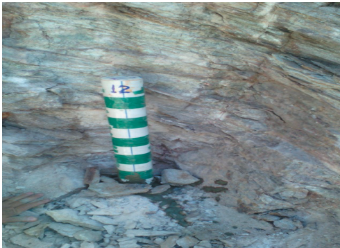
Fig. 1: Construction of Nuclear Track Tubes
