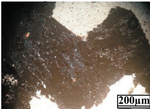
Fig. 14: Euhedral crystal of perthite, syenogranite, XPL
