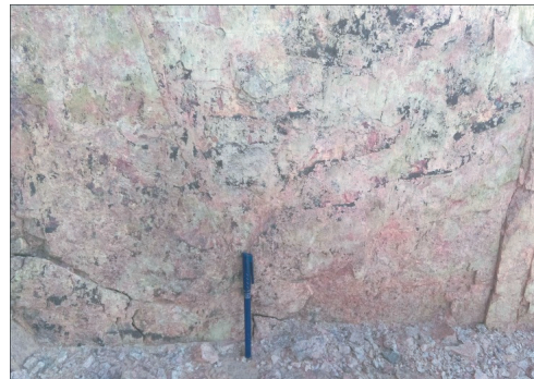
Fig.9: Close up view, showing hematitization, chloritization and kaolinization along fracture surface in younger granites, W.Umm Nafie area
