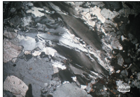
Fig. 10: Photomicrograph shows highly deformed Qz crystals as well as fragmented grains due to the high applied stresses, XPL
