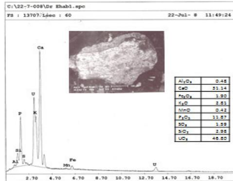
Fig.7: SEM backscattered image and EDX analyses for the separated meta-autonite
