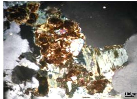
Fig.3: Iron oxides surrounded zoned zircon in chlorite, XPL
