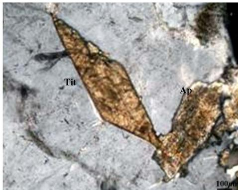
Fig.6: Sphene (Tit) and apatite (Ap) in quartz, XPL
